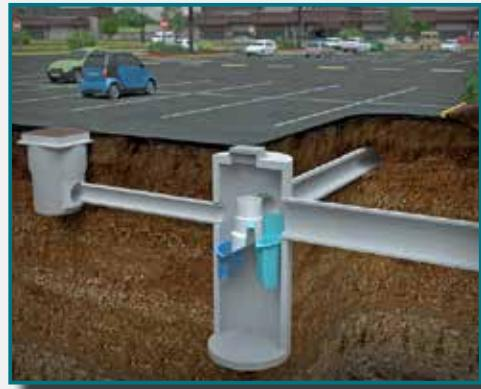
Contaminated stormwater runoff enters the inlet chute from a surface grate and/or inlet pipe. The inlet chute introduces flow into the chamber tangentially to create a low energy vortex flow regime (**magenta arrow**) that directs sediment into the sump while oils, floating trash and debris rise to the surface.
